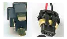
If installing on H4 type bulb with the halogen high beam, you will need to remove the high beam terminal pin from the above H4 3prong connector and manually stick it into your bikes harness. Next, you will have to wire the halogen high beam ground to the back of the relay ground wire. Without doing this your halogen high beam will not function. The high beam halogen wires are the thinner wires.
